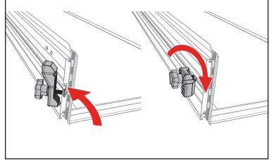
Set the cover (A) in the folded position on the side rails R (B & C) towards the cab of the truck. Confirm the cover is evenly spaced between the rails.
