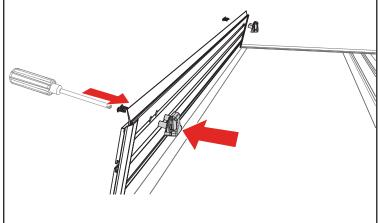
Confirm the retainer clamps (D) are positioned around the 9 side rails (B & C) correctly as shown below. Tighten the retainer clamps by turning them clockwise until the lock washer
