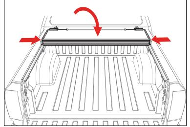
Attach the drain tubes (H) to the front of the side rails 5 (B & C) to allow water to be diverted out of the truck bed via the rail. Drill a 5/8" hole in the top corner of the wheel well as shown in the CAUTION Step (location 1), then run the opposite end of the drain tube through the 5/8" hole.
