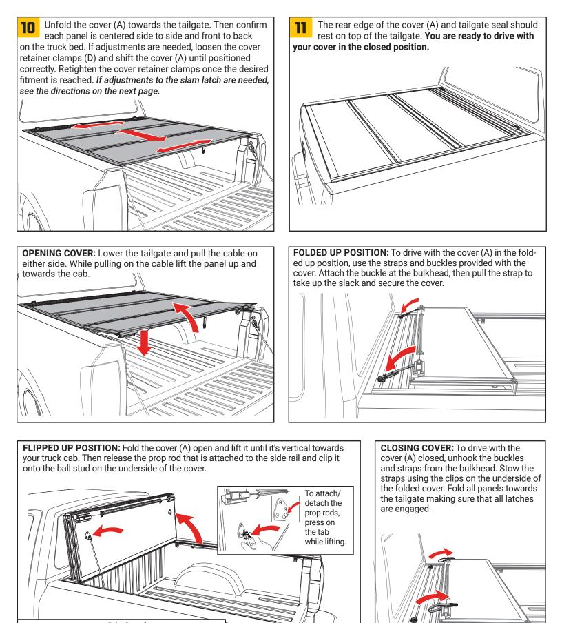
Before flipping cover (A) in the up position make sure to stow the straps using the clips on the underside of the folded cover.
