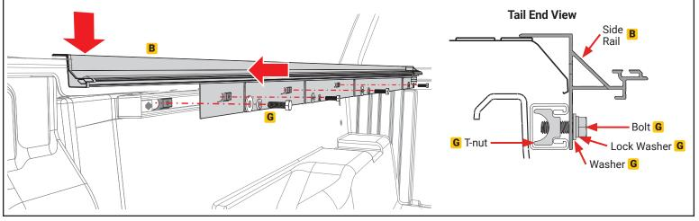
4 When you get the driver side rail (B) and the T-nut kits (G) lined up you can now tighten the bolts while you are applying downward pressure to the rail. A second set of hands may help. Repeat on the opposite side using the passenger side rail (C). Tighten all clamps to 10 ft/lbs of torque with a 1/2" wrench or socket. **Caution: Do NOT overtighten!**
